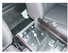
Attach "L" bracket mounting leg (#9) to rear floor filler panel (#6) using ½-20 x ¾" hex bolts and serrated nuts.
